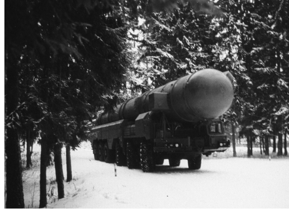
The RSD-10 Pioneer/SS-20 Saber Soviet intermediate-range ballistic missile (IRBM) with a nuclear warhead, first deployed in 1976. (I. Baskakov/Sputnik via AP)
