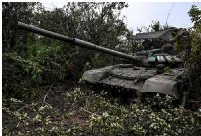
Destroyed Russian tank with cage armor, Kharkiv 2022. Russian armor modifications continue to evolve as the war goes on. (Photo by Juan Barreto/AFP via Getty Images)
