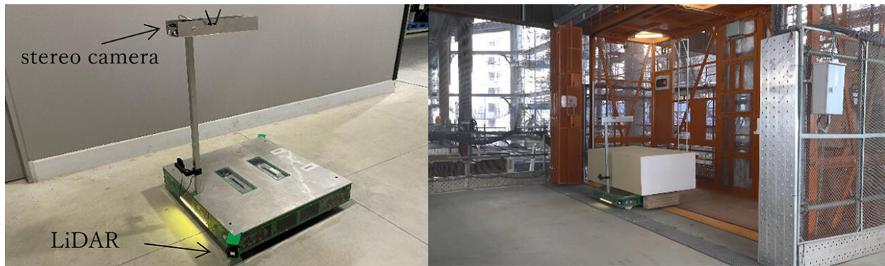
Obayashi's Low-Floor Automatic Guided Vehicle (left) Enters a Construction Elevator (right)
