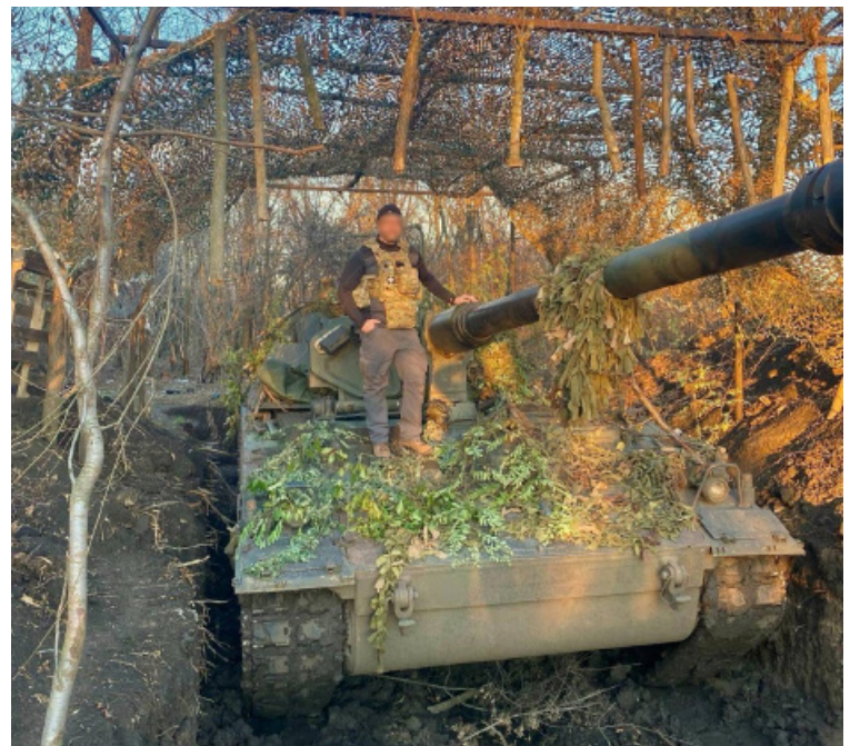
Example of a Ukrainian Panzerhaubitze 2000 self-propelled artillery piece parked in anti-drone shelter. (November 2023. Orikhiv-Tokmak direction.)
