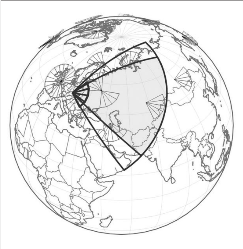
Figure A11. Zone covered by the identification and tracking EMR radar in the Czech Republic
